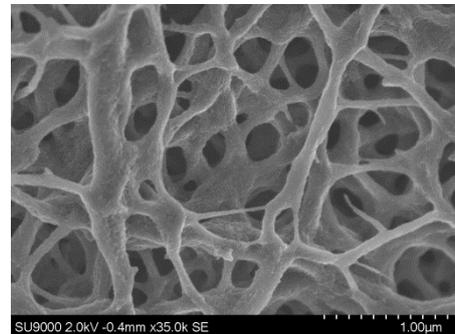
Figure 1: Micrograph of a highly porous carbon fiber fleece.
