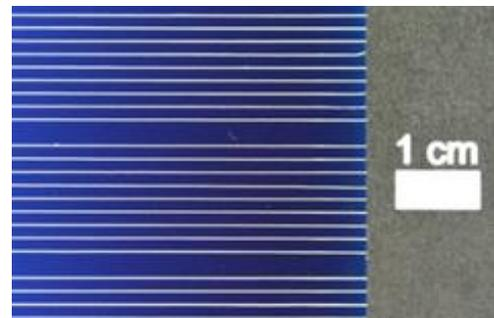
Figure: Deposition of fine silver electrodes on a silicon wafer using a dispenser system with 50  $\mu\text{m}$  nozzle diameter [Fraunhofer ISE, Freiburg].
