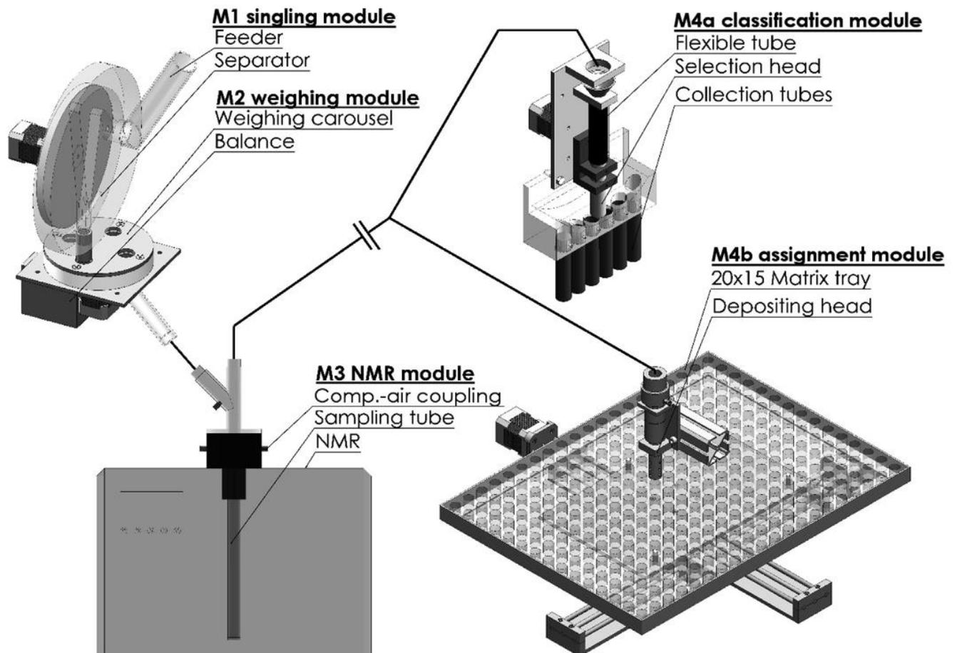
Figure 4: Schematic representation of all five functional modules [University of Hohenheim].
