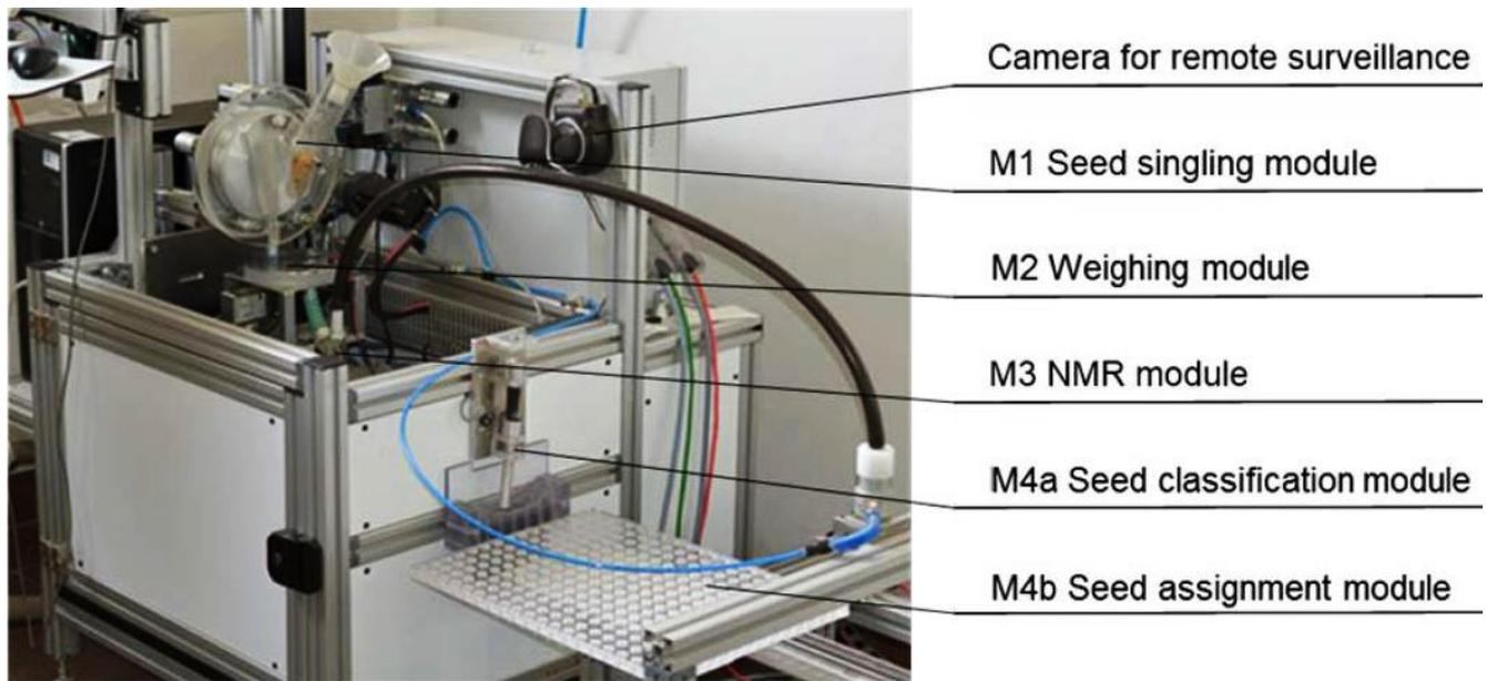
Figure 1: Overview of the invention with five functional modules with M1 for removing individual seeds from a bulk of seeds, M2 for weighing each seed, M3 for obtaining NMR measurements of seed oil mass, and either M4a for sorting individual seeds into predefined classes based on oil content or M4b for placing individual seeds in cells of a matrix tray to retain individual seed data [University of Hohenheim].
