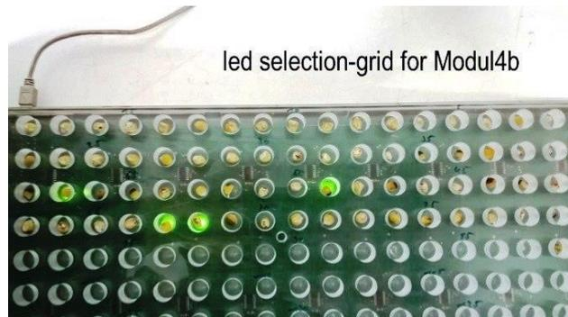
Figure 3: Close up of the matrix tray of Module 4b. Here, a bulk of seeds was phenotyped by the high-throughput platform for oil content and placed in individual cells of the tray with help of a computer-controlled X-Y table. Cells in the tray illuminated with green LEDs are the individual seeds meeting the selection criteria (defined by the user using a simple graphical interface for control software on the integrated computer) [University of Hohenheim].
