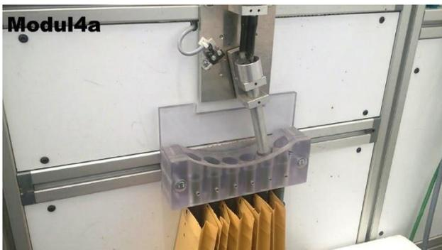
Figure 2: Close-up of the Module 4a for sorting a bulk of seeds into different classes. Here, each seed bag represents a different fraction of seeds based on oil content. The first class with lowest oil content contains mostly embryoless seeds, while the next two fractions with lowest oil content contain almost exclusively haploid seeds. In contrast, the highest oil fraction contains almost exclusively diploid seeds [University of Hohenheim].
